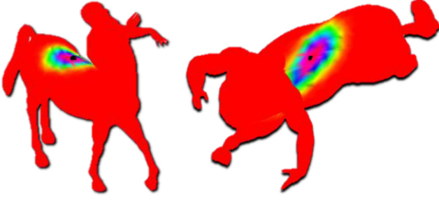
Figure 4: Anisotropic heat kernel centered at a (black) seed point on a coarse triangle mesh.
