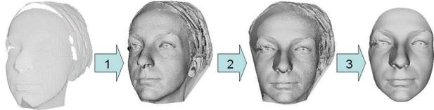
Figure 1. The various stages of the pre-processing. From raw point cloud to Delaunay triangulation (1), to pose-normalized mesh (2) and finally to cropped and smoothed mesh (3).
