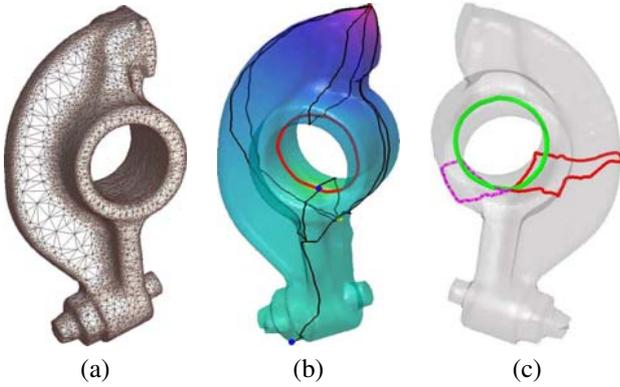
**Figure 7. (a) Input surface; (b) quasi Morse-Smale complex and longitude (red curve) of an irregularly sampled surface. (c) Generators: the meridian is the longest loop (red curve) belonging to the iso-contour of the saddle.**
