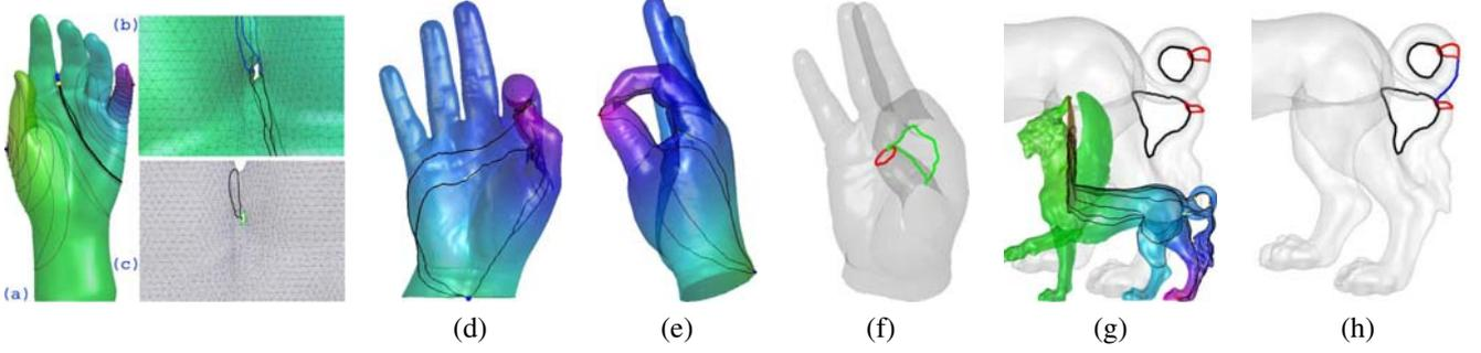
**Figure 11. (a) Quasi Morse-Smale complex, (b) saddle points, iso-contours, and (c) generators of a tiny handle. (d-e) Quasi Morse-Smale complex and (f) topological generators of a 1-genus surface. (g) Quasi Morse-Smale complex, handle generators of a 2-genus surface, and (h) final cut-graph.**
