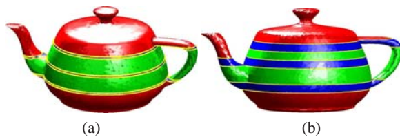
Figure 9: (a) Minimal decomposition with respect to the height function, and (b) adaptive segmentation induced by the parameterization distortion.
