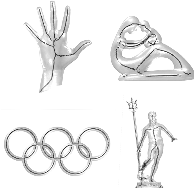
Figure 5.14: A gallery of point clouds obtained back-projecting 2D symmetry points with the accurate method. Only occlusion-free locally unique symmetry points have been considered. This method can generate almost noise-free point clouds for many different kinds of objects. For each model in the figure contours have been gathered by rotating around the most important axis given by the PCA.
