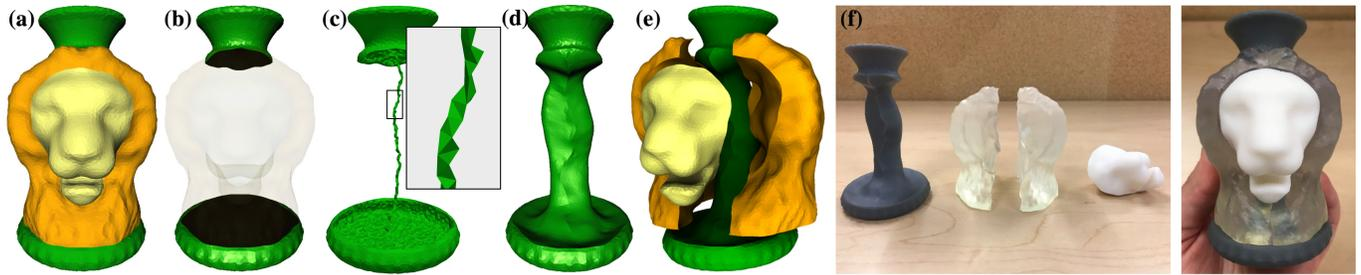
Fig. 11. Multi region part processing: (a) input surface; (b) two regions having the same *green* attribute; (c) tetrahedra affiliated with the green attribute after MST calculation; (d) single part formed out of the two merged green regions; (e) whole object decomposition; (f) printed parts and assembled object.
