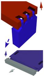
were not the axis-aligned ones that a human observer would predict (see inset). Specifically for the bench, Surface2Volume extracts the side part downwards and to the left, and extracts the table's side along a forward-left diagonal. Both computation and fabrication confirmed that these directions indeed enable assemblable partitioning.
