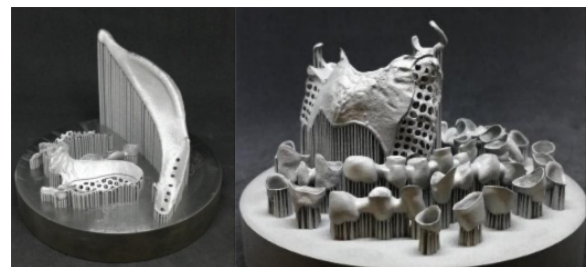
Figure 1: Based on the list of orders and their priorities, the same building platform may be filled differently. On the left, the denture (sheet) is an urgent order, hence it is placed horizontally for fast production. On the right, the same part is placed vertically so that more parts can be produced in the same overnight session.
