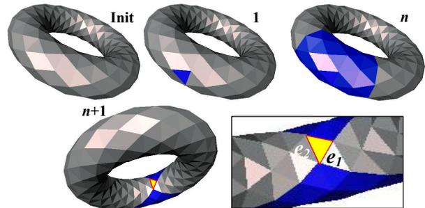
**Figure 3: Example of depth-first visit starting from a seed face and tagging of an  $S$  triangle.**
