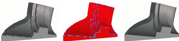
Figure 4: From left to right: original; smooth regions detected; sharpened model.
